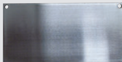
After 192 hours in a humidity cabinet, the metal coupon treated with Z-ROD Synthetic Motor Oil showed no signs of rust or corrosion.
