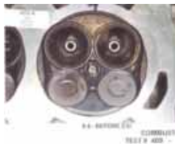
Picture F - Combustion chamber before P.i. treatment
