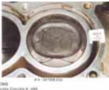
Picture I - Piston after P.i. treatment
