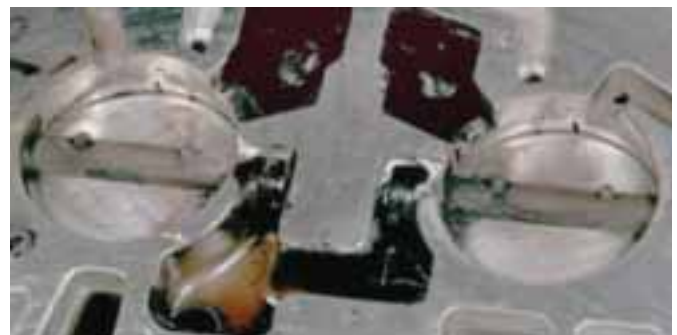
Picture K - Carburetor plates after P.i. treatment
