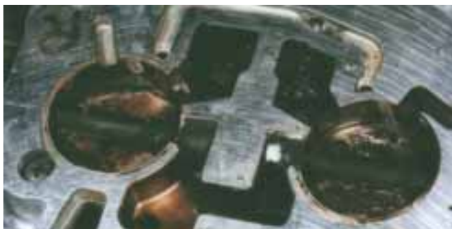
Picture J - Carburetor plates before P.i. treatment
